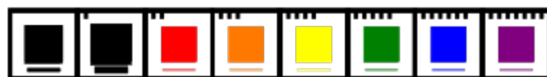
Figure 8.7: Symbols for the layers have little line segments to denote the layer number, and show the line width, fill colors and stroke colors in the border and fill of squares.
